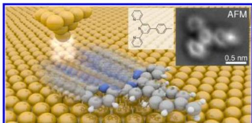
From [2]. Displacement under an electric field, generated by an STM tip, of a molecule that participated in the 2017 NanoCar Race[3]. Inset, image of the molecule obtained by atomic force microscopy.
